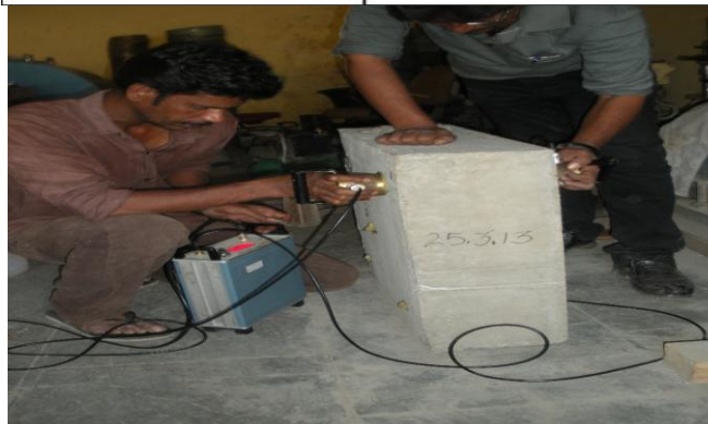
Fig.2. Conducting UPV on slab
